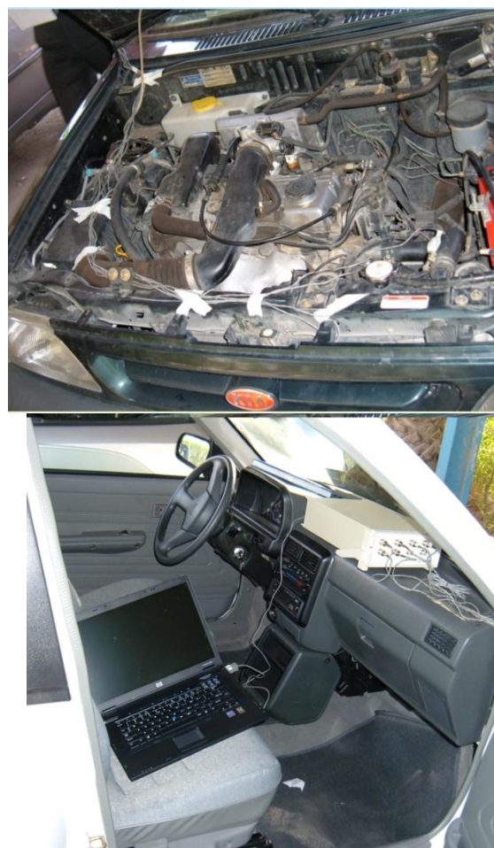
Figure 7: The data acquisition system and temperature sensors
