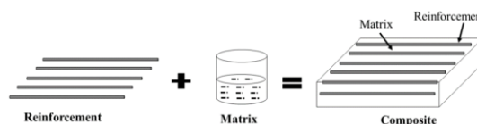
Figure 2 Schematic of FRPs
